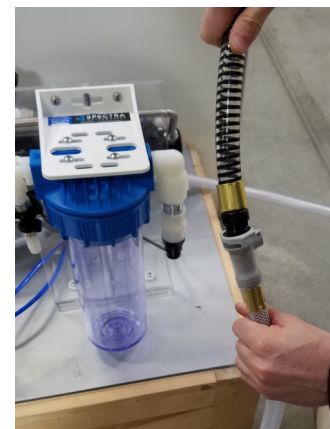
Removing hose to sea strainer from the “to strainer” pigtail.
