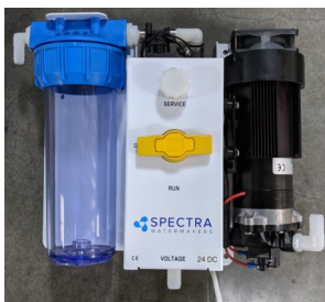
Service valve OFF, in FLUSH position
